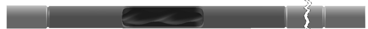
SHOT - SLIMHOLE: STATOR WITH BOX OR WELDED BOX CONNECTION; ASSEMBLY OD NOT LARGER THAN STATOR TUBE. WHEN ORBIT TUBE IS REQUIRED FOR HELIX OR ROTOR HEAD ROTATION. SAME AS FLOT WITH FURTHER REDUCED OD.
