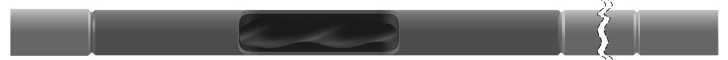
FLOT - FLUSHLINE: STATOR WITH BOX OR WELDED BOX CONNECTION; ASSEMBLY OD NOT LARGER THAN STATOR TUBE. WHEN ORBIT TUBE IS REQUIRED FOR HELIX OR ROTOR HEAD ROTATION.
