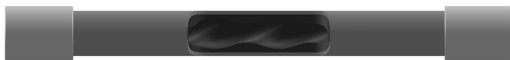
STD - STANDARD: STATOR WITH PIN THREADS; ASSEMBLY OD COLLARS LARGER THAN STATOR TUBE.
